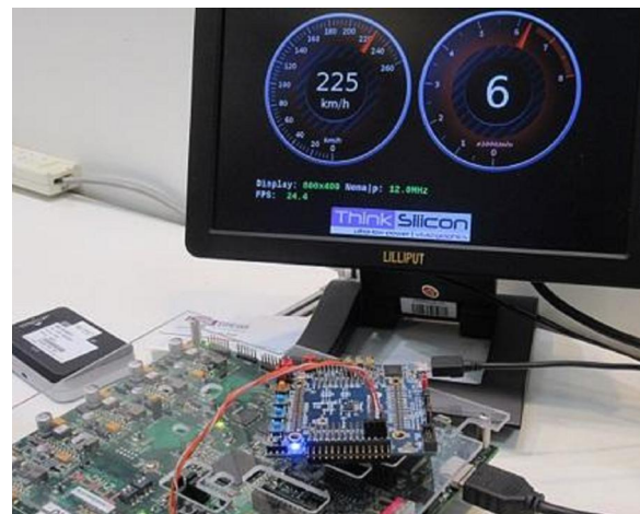
Think Silicon's Nema p (pico) is designed to build 2D display applications
